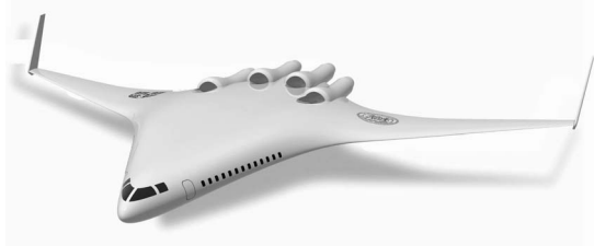
Fig. 2 A 3-D rendering of a candidate Silent Aircraft airframe and propulsion system, taken from [11]
