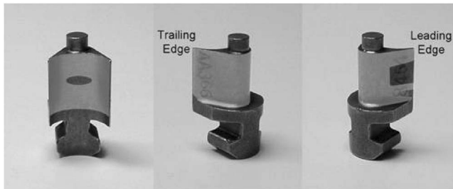
Fig. 13 First rotor dirt patterns observed during a field inspection (mapped on a new blade for clarity)
