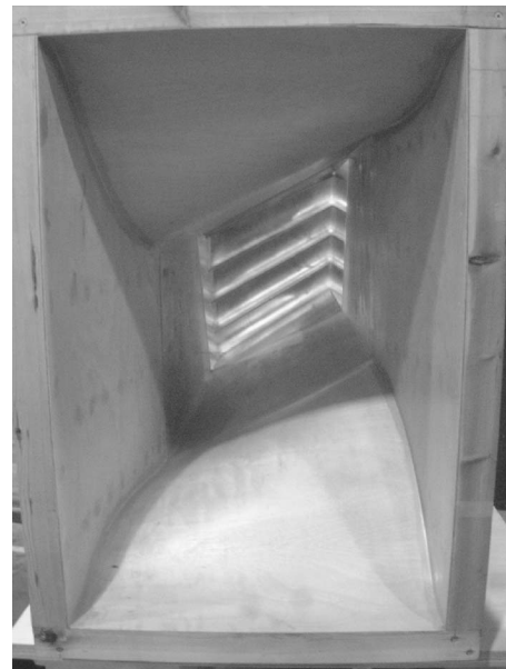
Fig. 14 Photograph of the inlet contraction for the swept cascade
